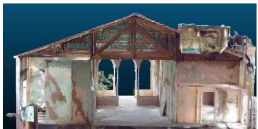
3D Model and 3D sections by Laser scanning
