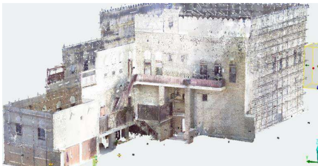
Point clouds Laser scanning output
