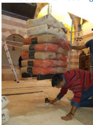
Load Test process where the white Baghdadi ceiling is seen at the left photo
