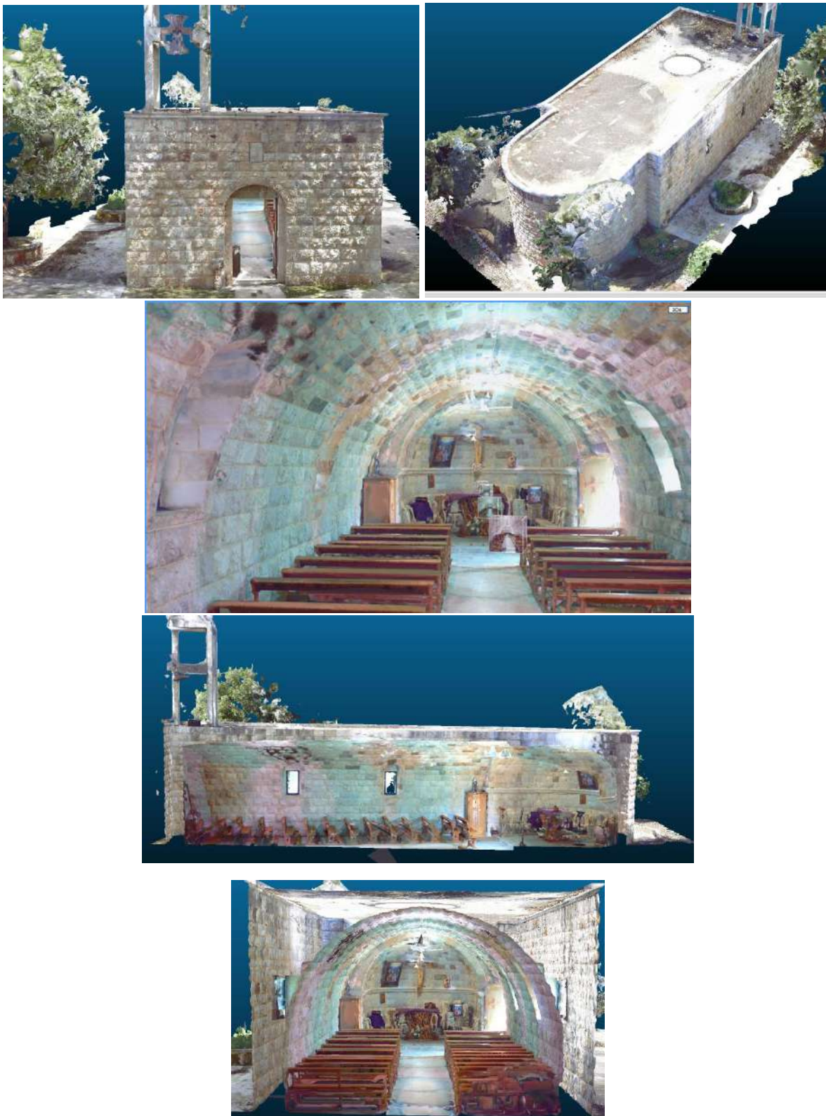
3D Model and sections by Laser scanning
